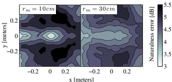
**Fig. 7:** Average naturalness error as a function of user position for two different microphone array radii.
