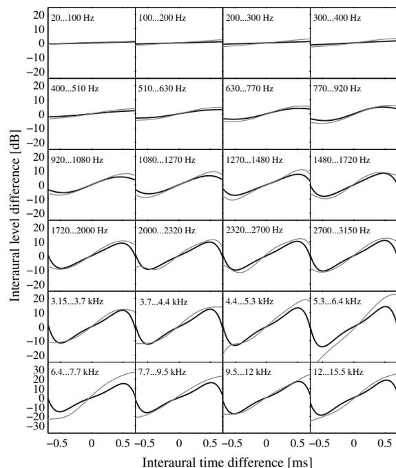
**Fig. 3:** Comparison between the naturalness functions  $F_i$  obtained with our auditory model (black lines), with the ones given by [4] (grey lines) in 24 critical bands.
