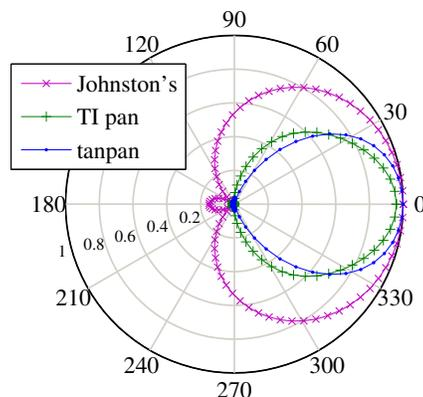
**Fig. 2:** Comparison between the different directivity patterns analysed in this paper.
