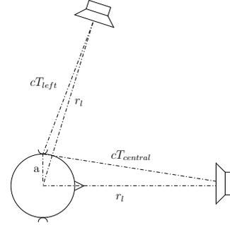
**Fig. 6:** Distances between left and central loudspeakers to the left ear.
