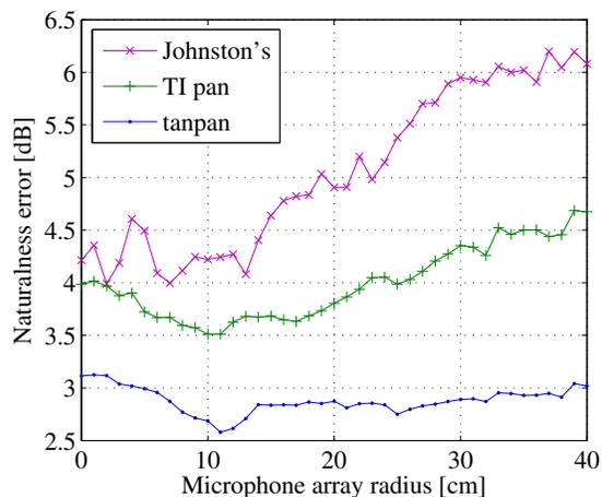
**Fig. 4:** Naturalness error as a function of the microphone array radius  $r_m$ . The user position is  $x = 0, y = 0$  and heading  $\phi = 0$ .
