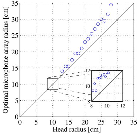
**Fig. 5:** Optimal microphone array radius in terms of naturalness as a function of listener’s head radius.
